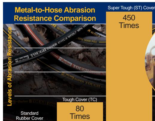
Results from the ISO 6945 metal-to-hose abrasion test show that Tough Cover and Super Tough cover hoses offer significantly greater abrasion resistance than standard rubber cover hose.
