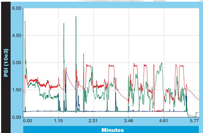
*Pressure spikes can occur during machine operation in an instant. They can occur so quickly in fact, that standard glycerin filled gages will never detect them. Using a pressure diagnostic system like Parker's Senso Control can help detect how often and how drastic these pressure spikes are.*
