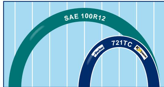
721TC Extreme hose has one-half the minimum bend radius of SAE 100R12 hose.
