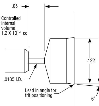
Pressed in frit eliminates movement of frit under pressure or disassembly.
