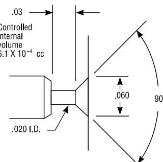
Drop in frit allows accessibility for micron changes and cleaning
