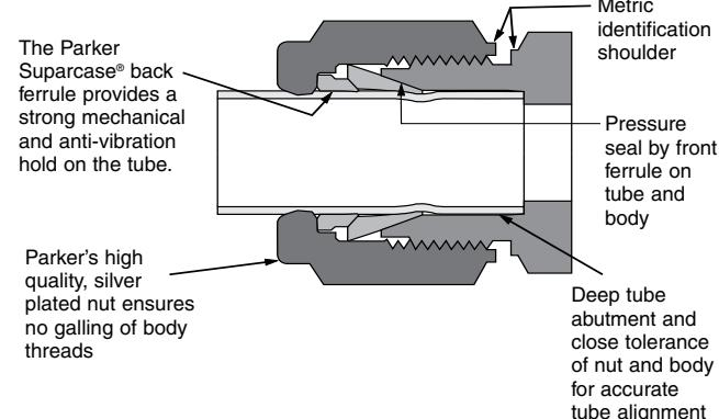
Parker Instrumentation Tube Fittings are supplied complete and ready to use. The ferrule(s) swage onto the tube as it moves down the body seat creating a pressure/vacuum-tight seal on both tube and body by the interface pressure and surface finish of mating components. The Parker Suparcase® ferrule (back-ferrule only on A-LOK®) creates a strong mechanical hold on the tube.
