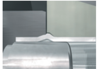
The inner contour also gets slightly deformed but remains smooth and unrestricted for good flow characteristics
