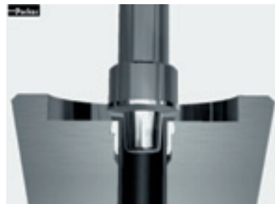
The front surface is continuously rolled and compressed. From the inside, the tube surface is slightly expanded to clamp the sleeve
