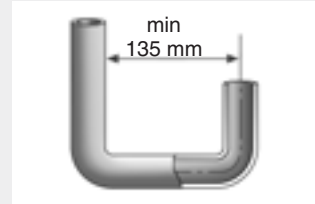
● Minimum clearance of U-shape bends
